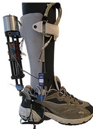
Figure 2-19 MIT's Variable Impedance AFO (adapted from [90]).
